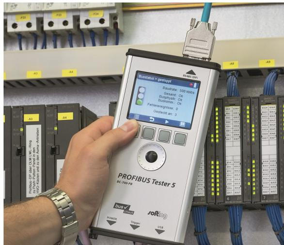
troubleshooting tool for comprehensive testing of PROFIBUS segments during operation and can now also be used for cable testing. The device is battery powered which guarantees maintenance- and commissioning engineers the highest level of mobility in the field.
